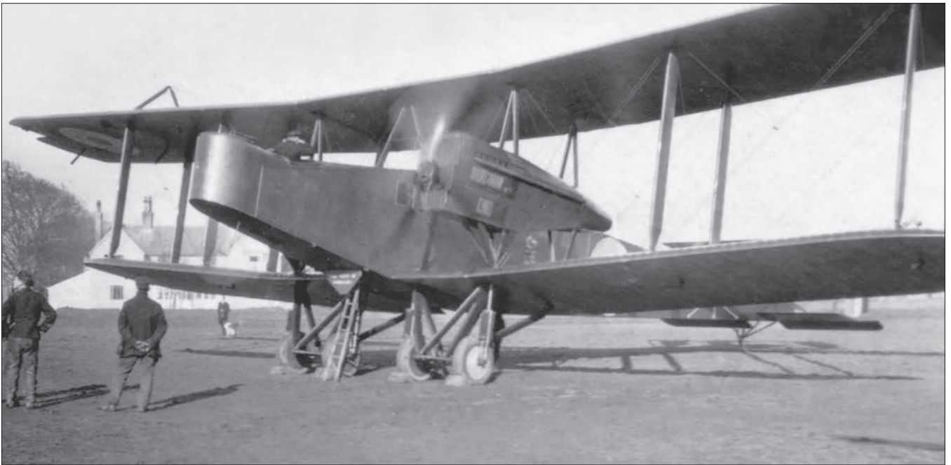
Testing the engines of a Handley Page O/100.
