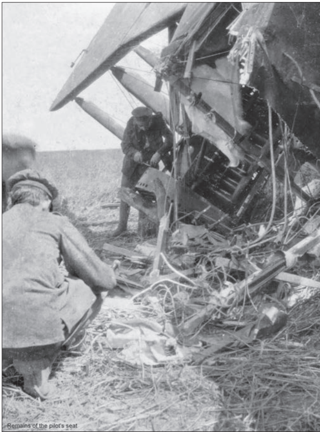
The wrecked nose area of C9646, with the remains of the pilot's seat.
