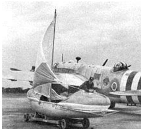
It is a Vickers Warwick ASR Mk 1 of 280 Sqn. Coastal Command, RAF Langham, Norfolk in October 1944. It carried an Uffa Fox designed, fully equipped lifeboat under the belly of the aircraft. It was a little bigger than a Wellington and was in fact a slightly earlier design.
